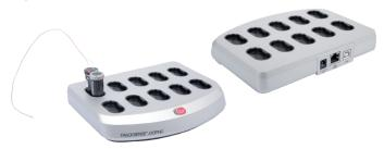
The LyoPro 10-slot multi reader station also has a completely new design to accommodate for the new data logger. Besides handling up to 10 data loggers at a time, the data transmission is done through Radio Frequency (RF), allowing for a much higher speed. The interface to PC is done by either USB or Ethernet (LAN), while the reader station is equipped with an IP address shown in the window in the bottom plate.
