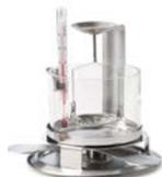
Dedicated kit for determining the density of solid and liquid substances with the built-in application.
