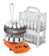
Work-Up Station for parallel or sequential work-up of 12 samples, using filtration, phase separation, liquid/liquid extraction or SPE.
